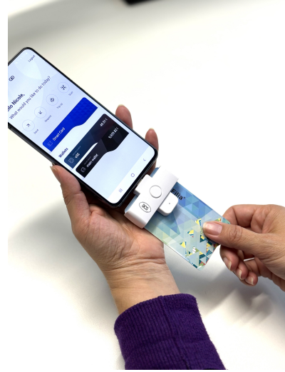
Figure 6: Phone with attachable card reader, allowing for card-to-card payments without special devices
